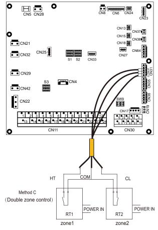
There are three methods for connecting the thermostat cable (as described in the picture above) and it depends on the application.
