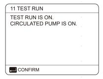
When circulation pump running is turned on, all running components will stop. 60 seconds later, the SV2 will be on, 60 seconds later PUMPI will operate. 30s later, if the flow switch checked normal flow, PUMPI will operate for 3min, after the pump stops 60 seconds, SV2 will be off. 60s later the both PUMPI and PUMPO will operate, 2 mins later, the flow switch will check the water flow. If the flow switch closes for 15s, PUMPI and PUMPO will operate until the next command is received.
