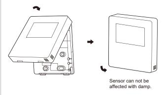
Correct install the back cover and firmly buckle the front cover and back cover, otherwise will make the front cover drop off.
